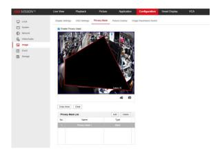
Third Stream support NPQ (Smooth Streaming). When Smooth Streaming is enabled, functions such as, variable bitrate, MJPEG, SVC, EPTZ, and Target Cropping, are not supported.
