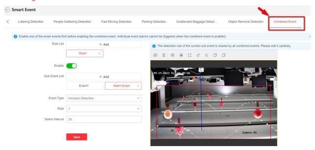
3) Support configure alarm interval (1~60s), default value is 30s. It is the maximum interval between different perimeter events triggered within a combined alarm.
