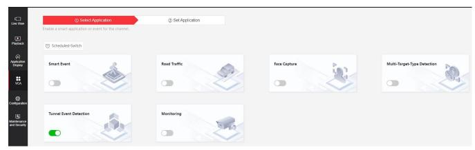
On Tunnel Event Detection mode, the camera supports fallen object detection, pedestrian detection, parking detection, congestion detection and construction detection.
