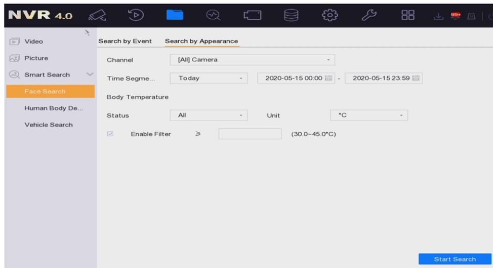
3) Support local and 4200 to search face pictures according to body temperature status and temperature range, and support to display search results in specified temperature units.
