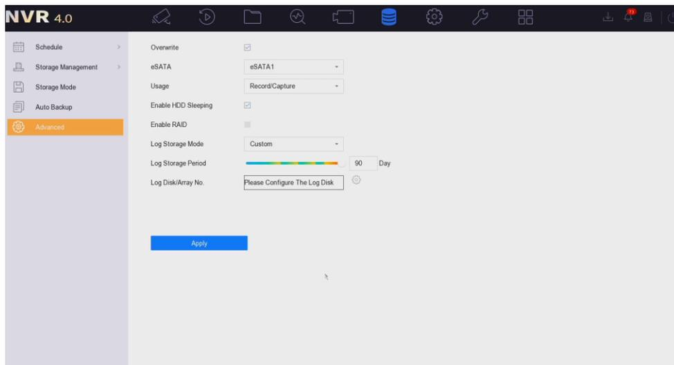
1) Designate one HDD as the log HDD to store logs, and add log HDD configuration and management.
