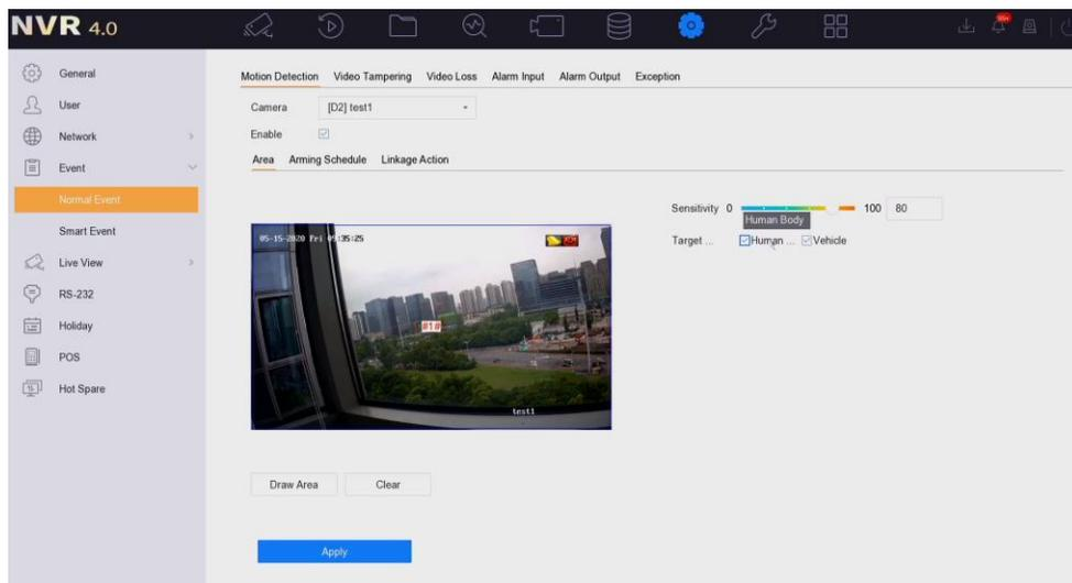
1) Support IPC with motion detection 2.0 function, the specific model of IPC is DS-2CD20 (23 / 2T / 26) 2 (4/8) 6G2-I / SL, such as: DS-2CD2026G2-I / SL. The firmware version of IPC is required to be V5.5.130 and later.
