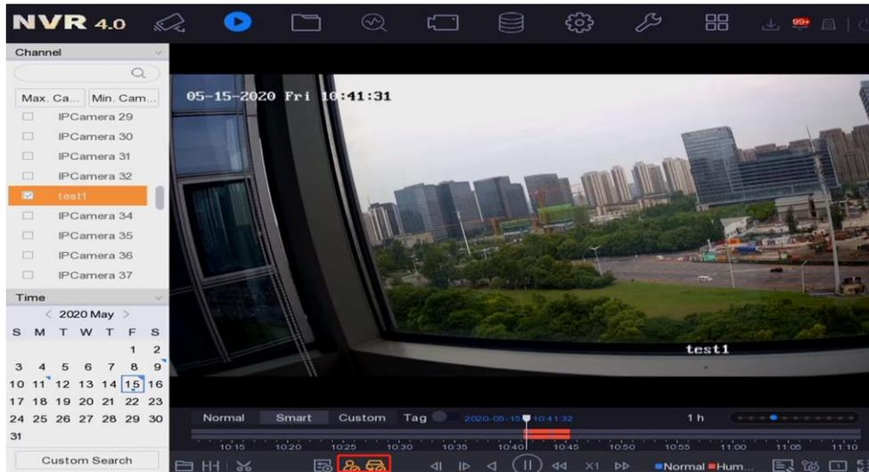
3) The smart playback interface for local playback and the remote ordinary playback interface add the option of human body-vehicle filtering. After checking, the human body-vehicle video information will be marked in red on the progress bar.
