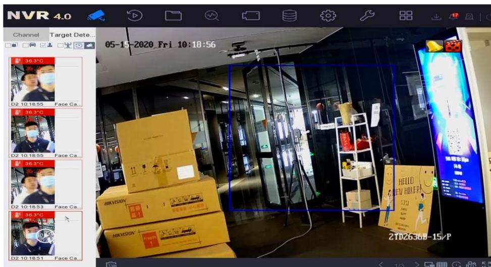
1) Support local target detection interface and 4200 to display real time face temperature alarm, abnormal temperature display red background, normal temperature display green background.
