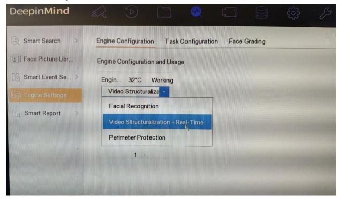
2) Then go to Smart Analysis > Smart Event Settings > Video Structuralization and click the Enable Multi-Target-Type Detection and configure Arming schedule, Linkage action
